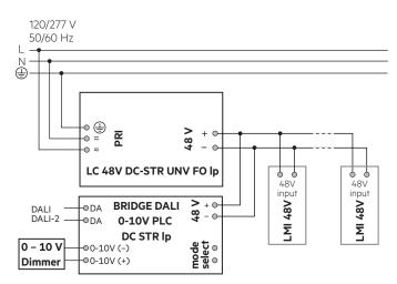
To use dimming functionality use dimmable LMI LED drivers with "DIM" in the product name.
