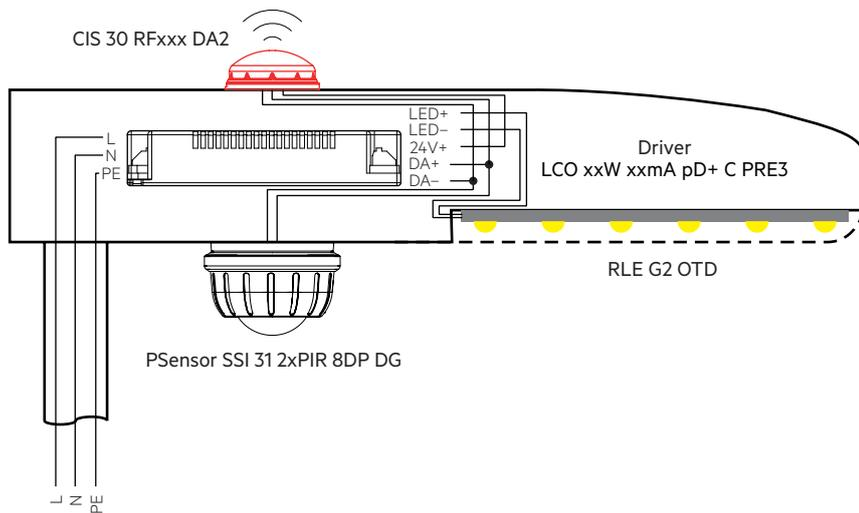
The RFNode supports the Zhaga connectivity standard for Plug&Play luminaire extensions. This allows a toolless and flexible integration in luminaires.
