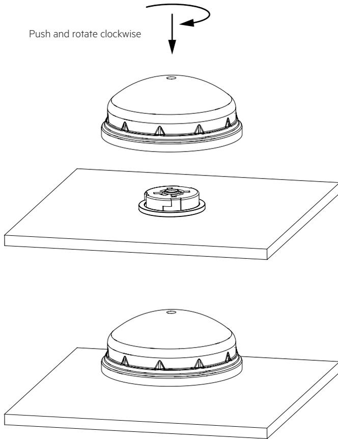
**!** The RFNode must lock. Make sure that the dust and dirt protection, is not bent, no foreign parts between the seal and the fixture housing are located and that the protection fits the fixture.
