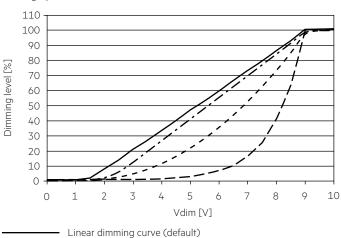
Dimming profiles programmable via NFC.
